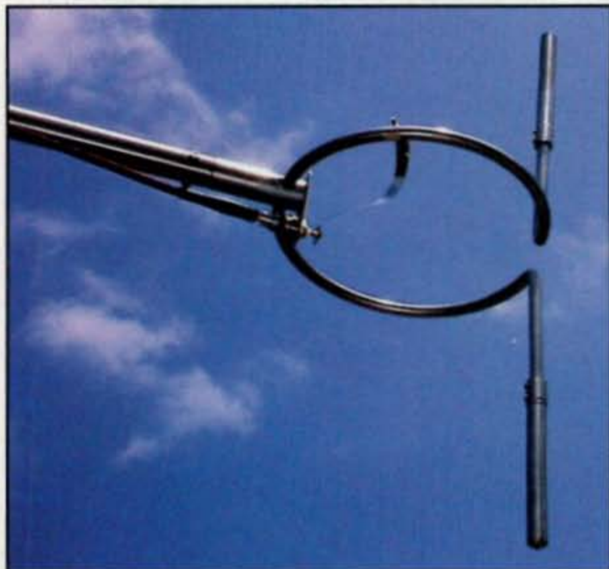
Photo A— The ring-stub circularly polarized antenna.
