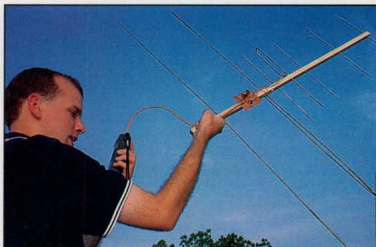
Photo F— 435/145-MHz Cheap Yagi for low-Earth-orbit satellites. Watch for details in an upcoming column.
